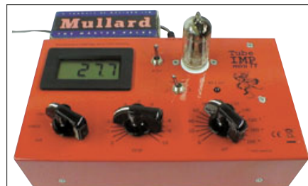
PHOTO 2: Tube Imp testing Mullard ECC83.
