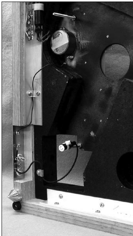
PHOTO 3: Bottom view of the turntable base with the new connector plate installed. The rear aluminum angle bracket is shortened to make room for the connector plate cutout.
