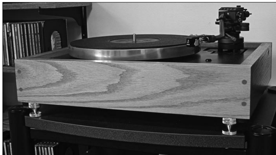
PHOTO 5: The upgraded belt-driven turntable. Dayton adjustable brass cones replace the old turntable sub-base.
